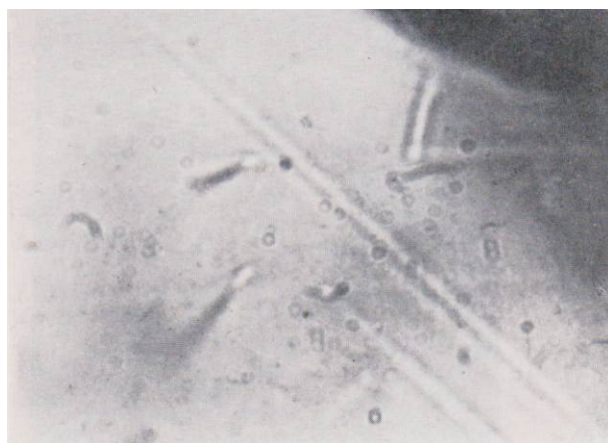
Figure 1. Microphotograph of ^{238}\text{U} spontaneous fission-fragment tracks in a sphene grain separated from ancient ashes left by Peking Man in Layer 10 of Locality 1 in Peking Man Site at Zhoukoudian, Beijing. The sphene grain was completely annealed by Peking Man when they were making fires. No crowded tracks formed before firing was left in the completely annealed grain. Only a few tracks formed after the firing made by Peking Man appear clearly on the surface of the grain. These tracks were used to date Peking Man ( 0.462 \pm 0.045 Ma in Layer 10 of Locality 1 in Peking Man Site).
