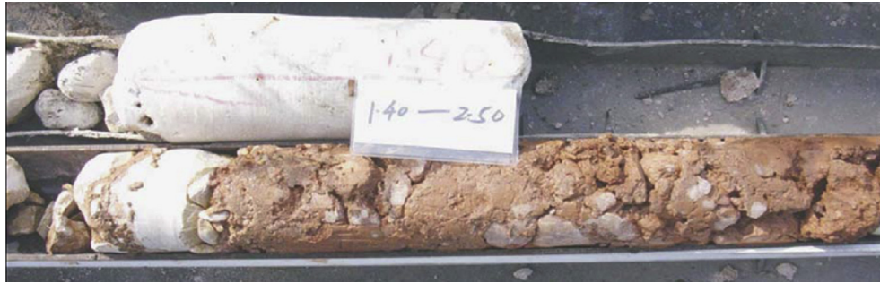
Fig. 4. Core from bore-hole S9. Note the contrast between solid limestone and a zone filled with brecciated clays.
